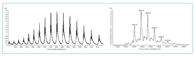
MS spectrum of deglycosylated ANTI-FLAG antibody following a 600 pg (4 fmol) injection on column. The deconvoluted spectrum on the right shows six different major glycoforms. Analysis was performed using HPLC-Chip/MS with 43 mm ZORBAX SB 300-C18 chip. (Agilent HPLC-Chip/MS and 6530 Accurate-Mass Q-TOF)
