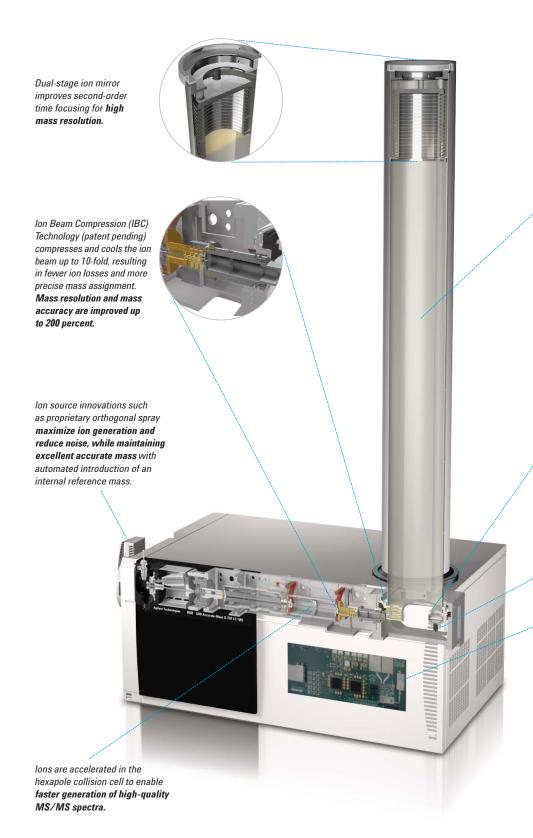
Proprietary INVAR flight tube sealed in a vacuum-insulated shell eliminates thermal mass drift due to temperature changes to maintain excellent mass accuracy, 24/7.
