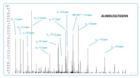
An MS/MS spectrum is shown for a peptide, ALIMDLEGLTGQIVK, from <u>Schizosaccharomyces pombe</u>. The average product ion mass accuracy was 2.3 ppm. All b- and y- ions from the peptide are shown with corresponding mass accuracy values. (Agilent HPLC-Chip/MS and 6538 Accurate-Mass Q-TOF)
