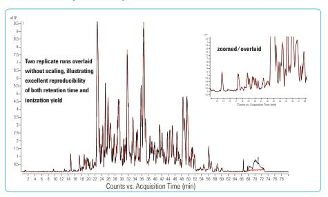
Overlaid chromatograms are shown for two replicate runs of a tryptic digest of an SEC fraction from a Schizosaccharomyces pombe sample. The results show the high level of reproducibility of both retention time and ionization yield. (Agilent HPLC-Chip/MS and 6540 Accurate-Mass Q-TOF)
