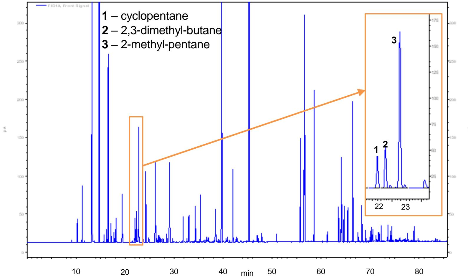
Agilent 7890GC with ICE-DOOR + SIM Multi Cooling Device, column: HP Pona (100m x 0.25mm x 0.2 $\mu$ m); carrier gas: H<sub>2</sub> (1ml/min); injection volume: 1  $\mu$ l; temp. program: 0°C for 10 min, 1.5°C/min to 60°C, 5°C/min to 120°C, 10°C/min to 240°C; detection: FID
