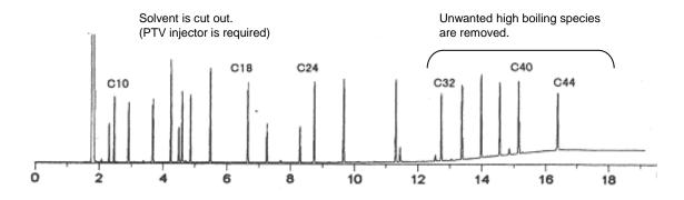
Detector contaminations are minimized by eliminating unwanted solvents such as TMS agent, etc. This is extremely useful in ECD and GC/MS experiments. Removing high boiling species results in significant reduction of analysis time and column baking time, leading to extended life of separation columns.
